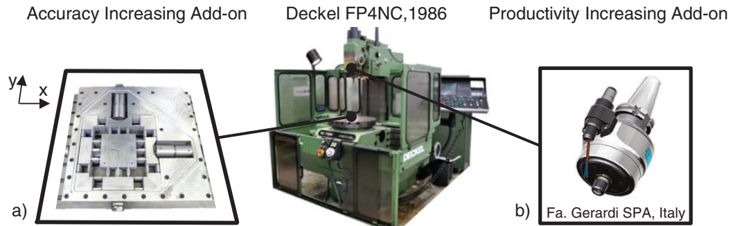
Fig. 1. Deckel FP4NC milling machine (a) accuracy increasing add-on; (b) productivity increasing add-on
