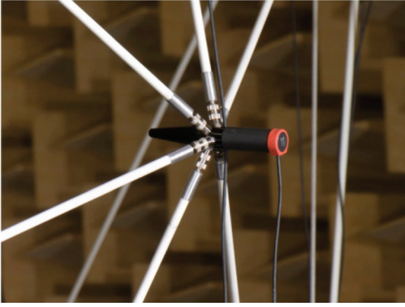
FIG. 4. (Color online) Supporting beam-structure (six beams) for one of the microphones.
