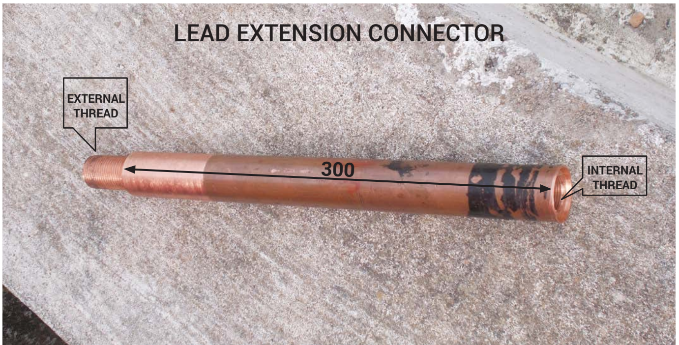
Figure 6. Copper extension piece showing suitably turned threads at both ends.
