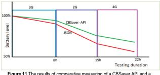
Figure 11 The results of comparative measuring of a CBSaver API and a classical JSON manner of transfer
