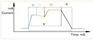
Figure 2 Segmented presentation of an energy profile of a REST request
