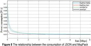
Figure 8 The relationship between the consumption of JSON and MsgPa schemes at different levels of compression
