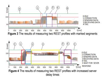
Fig. 4 represents a recorded profile of a test during which the time necessary for the server to process the request was drastically increased to 5 s in order to be able
