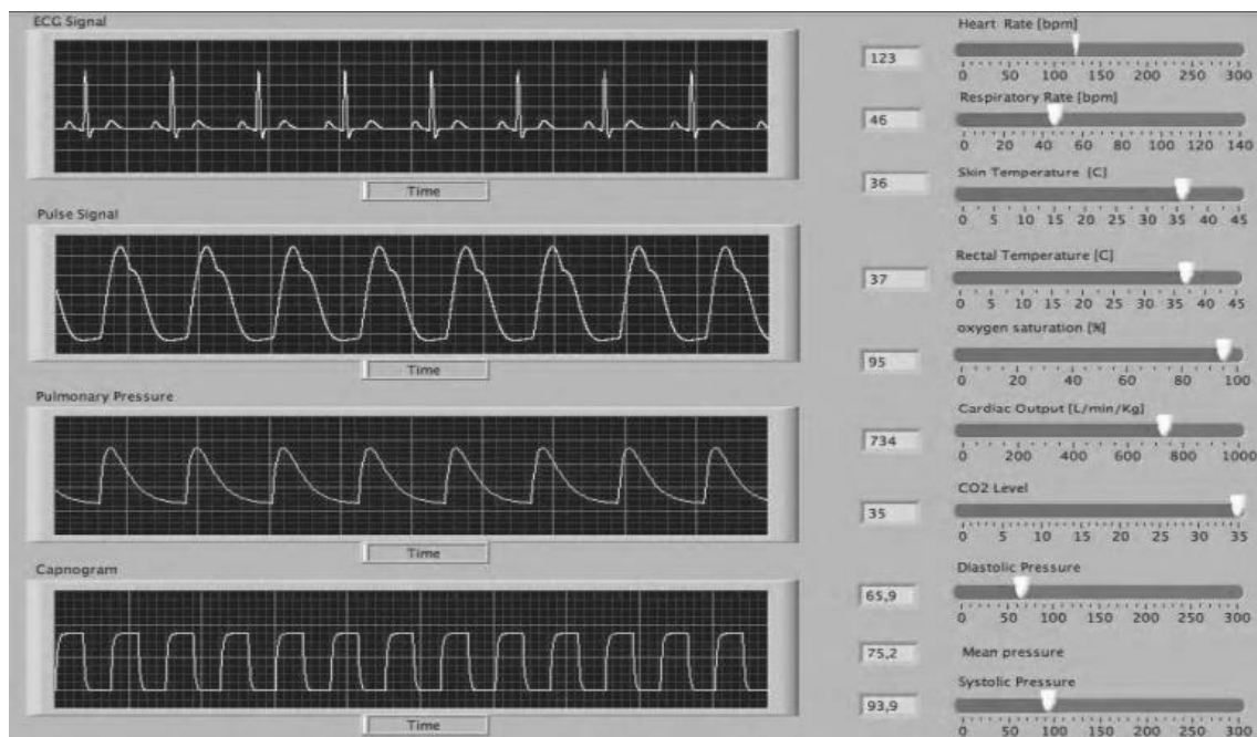
Figure 9. Existing ECG simulator without filtering and modeling noise.
