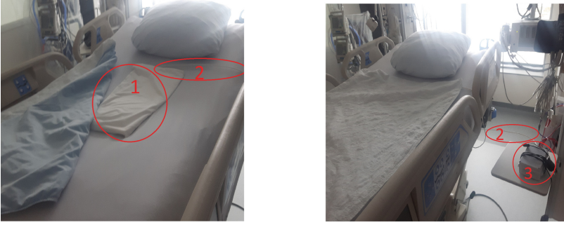
Fig. 4. Positioning of the smart mattress (1) and its acquisition box (3). On the left, we see the smart mattress (1) encased in a waterproof pillowcase. This is to protect it against standard biohazards present in a hospital as well as to meet the sanitary requisites of the hospital. On both images, we see the fiber optic cable (2) going from the smart mattress (1) to the acquisition box (3).
