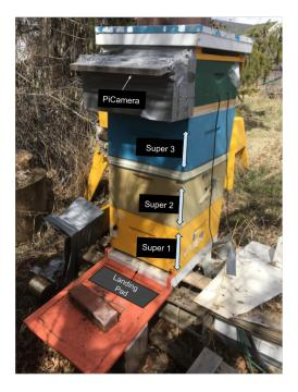
**Figure 1.** A BeePi monitor box on top of a Langstroth beehive that consists of 3 supers; the camera is protected against the elements with a specially constructed wooden box. More hardware details are available at [42,43].
