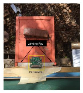
**Figure 3.** A closer look at the camera looking down on the landing pad. More hardware details are available at [42,43]. When the monitor is placed on the third super, as shown in the picture, the monitor's camera is  $\approx$ 85 cm above the landing pad and the camera's field of view in this picture is  $\approx$ 200 cm high and  $\approx$ 320 cm wide.
