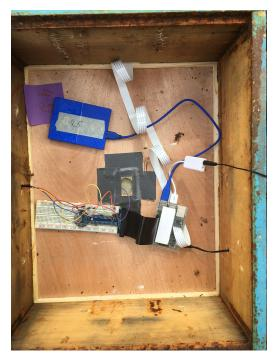
**Figure 2.** A BeePi monitor consists of a raspberry pi 3 model B v1.2 computer, a pi T-Cobbler, a breadboard, a waterproof DS18B20 temperature sensor, a pi v2 8-megapixel camera board, a v2.1 ChronoDot clock, and a Neewer 3.5 mm mini lapel microphone placed above the landing pad. More hardware details are available at [42,43].
