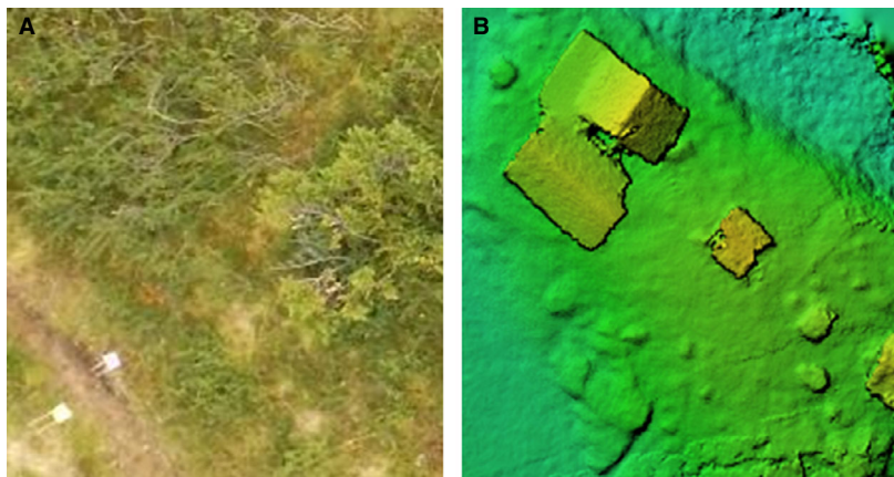
Figure 2. (A) 100% crop of the orthophoto resolution where the bare soil (bottom left side) can be distinguished from the vegetated areas. Juniper shrubs can be identified (upper half of the image) and (B) DSM of the cabins where the roofs are clearly distinct from the ground surface.
