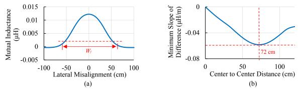
Fig. 3.11: (a) The effective zone for a given mutual inductance profile (b) Optimum operating zone selection for the double-coil system.
