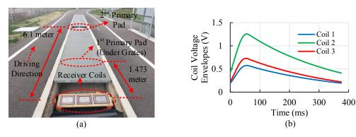
Fig. 3.21: (a) DWPT-VDS RC setup and primary coils installed in the road (b) The detected voltage envelopes of the RCs when the bus is moving at 24 km/h.
