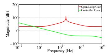
Fig. 5.18: Magnitude Bode plot of SC-converter openloop gain and controller transfer function.
