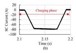
Fig. 4.41: (a) SC voltage  $V_{sc}$  and (b) SC current  $I_{sc}$  during the *charging phase* in V2G operation with bang-bang type control action of the *grid current controller*.
