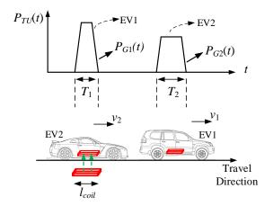
Fig. 2.6: The power profile at the TU input.
