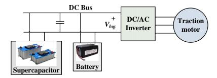
Fig. 5.5: Passive parallel structure of HESS.
