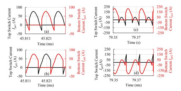
Fig. 4.47: The inverter switch currents in the systems without the buffering unit for (a) leg pa and (b) leg pb; the inverter switch currents in proposed system for (c) leg pa and (d) leg pb. Waveforms are taken during the rated 25-kW G2V power transfer.
