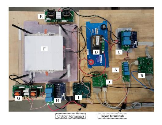
Fig. 4.60: Experimental setup for grid-side energy management.
