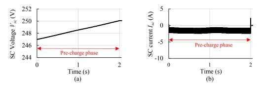
Fig. 4.30: (a) SC voltage  $V_{sc}$  and (b) SC current  $I_{sc}$  during the precharge phase.
