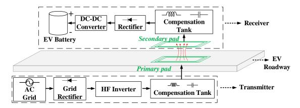
Fig. 2.1: A typical grid-powered DWPT system.
