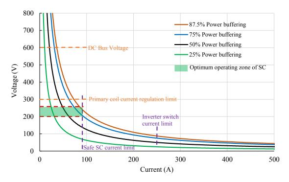
Fig. 4.7: Optimum operating region of SC unit.
