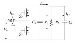
Fig. C.1: Boost converter circuit.
