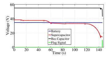
Fig. 5.25: Battery voltage, SC voltage, DC bus voltage and flag signal during dead-zone test with no DWPT.
