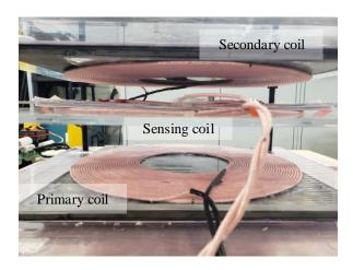
Fig. 4.57: Primary coil, secondary coil, and sensing coil of the experimental setup.
