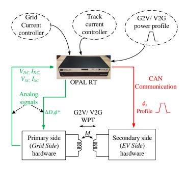
Fig. 4.49: System block diagram of the experimental prototype.
