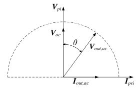
Fig. 2.15: Phasor diagram of voltage and currents associated with BWPT power transfer.
