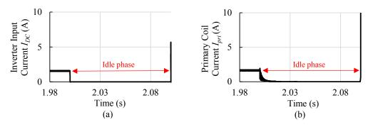
Fig. 4.31: (a) The grid current  $I_{DC}$  and (b) the primary coil current  $I_{pri}$  (RMS value) during the *idle phase*.
