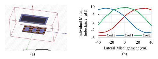
Fig. 3.14: (a) FEM simulation model of the three-coil detection system (b) Simulated lateral axis mutual inductance profiles.
