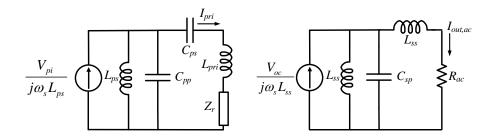
Fig. 2.13: Source-transformed primary and secondary equivalent circuit.
