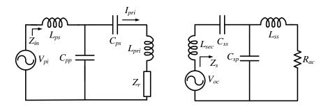
Fig. 2.11: The simplified equivalent circuit after coupling between primary and secondary coils is replaced by  $V_{oc}$  and  $Z_r$ .
