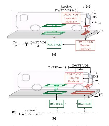
Fig. 3.2: System block diagram of (a) DWPT-RSDS (b) DWPT-VSDS.
