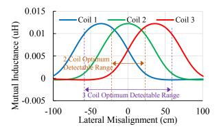
Fig. 3.13: Lateral mutual inductance profile for the three-coil system.
