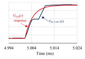
Fig. 4.15: Step response of  $G_{DM}(s)$  and  $V_{pi,1,rms}$  to a step change where  $T_{hi} = 120^{\circ}$ .
