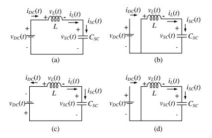
Fig. B.5: Inverter circuit during (a)  $0 < t < d_1(t)$  subinterval (b)  $d_1(t) < t < d_1(t) + d_2(t)$  subinterval (c)  $d_1(t) + d_2(t) < t < d_1(t) + d_2(t) + d_3(t)$  subinterval (d)  $d_1(t) + d_2(t) + d_3(t) < t < T_s$  subinterval.
