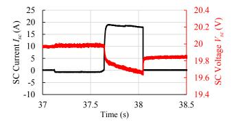
Fig. 4.73: SC voltage  $V_{sc}$  and current  $I_{sc}$  profile recorded by OPAL-RT during the *charging phase*.
