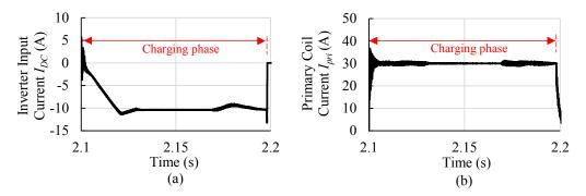
Fig. 4.38: (a) The grid current  $I_{DC}$  and (b) the primary coil current  $I_{pri}$  (RMS value) during the *charging phase* in V2G operation with FFFB type control action of the *grid current controller*.
