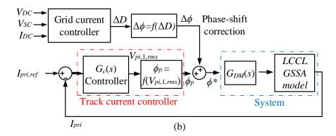
Fig. 4.12: (a) The block diagram of a track current controller (b) Combined system's block diagram with track current controller and the grid current controller.
