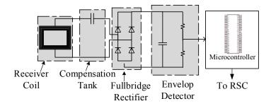
Fig. 3.4: VDS receiver circuitry.
