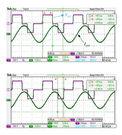
Fig. 4.71: Inverter output voltage  $V_{pi}$  and primary coil current  $I_{pri}$  during the charing phase.
