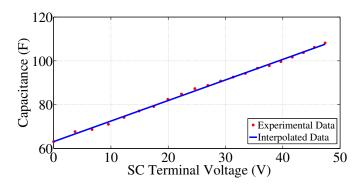
Fig. 5.3: SC characteristic curve.
