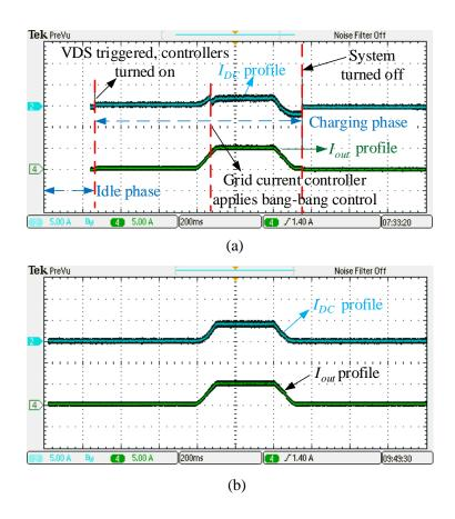
Fig. 4.72: Comparison of the inverter input current  $I_{DC}$  and output current  $I_{out}$  profile in the *charging phase* (a) with grid-side buffering (b) without the grid-side buffering.
