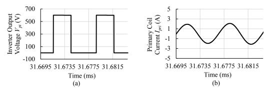
Fig. 4.28: (a) The inverter output voltage  $V_{pi}$  and (b) primary coil current  $I_{pri}$  waveforms during the *precharge phase*.
