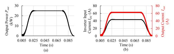
Fig. 4.24: (a) Output power  $P_{out}$  (b) inverter input current  $I_{DC}$  and inverter output current  $I_{out}$  for G2V charging operation.
