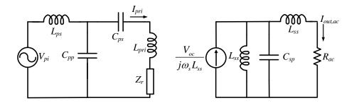
Fig. 2.12: Decoupled primary and source-transformed secondary equivalent circuit.
