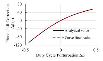
Fig. 4.22:  $\Delta \phi$  vs.  $\Delta D$  locus around the operating condition of  $\phi_p$  =60° and  $D_a$ =0.5.
