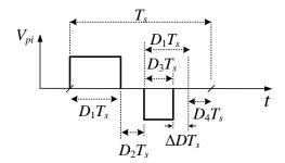
Fig. B.4: Single period of inverter output.
