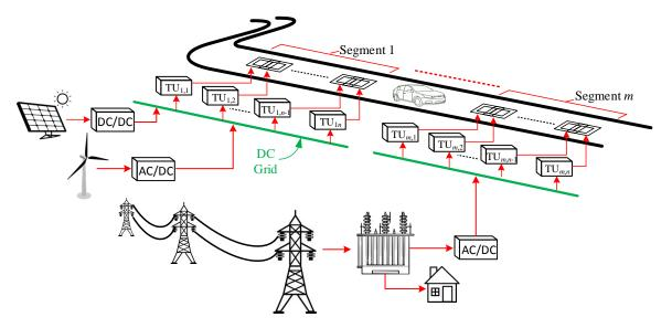
Fig. 2.3: Dynamic charging system at a large scale with illustrated sectional organization.
