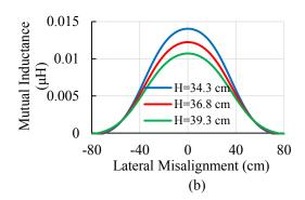
Fig. 3.8: Mutual inductance profile of a single-coil system for three different ground-clearances.
