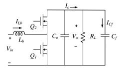
Fig. 5.16: Boost converter circuit.
