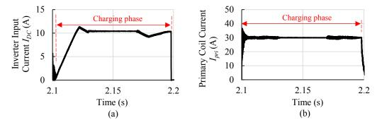
Fig. 4.33: (a) The grid current  $I_{DC}$  and (b) the primary coil current  $I_{pri}$  (RMS value) during the *charging phase* in G2V operation with FFFB type control action of the *grid current controller*.
