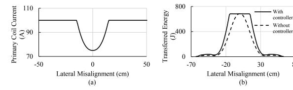
Fig. 3.24: (a) The primary coil current reference as a function of LTM (b) Energy-transfer comparison with and without the controller [1].
