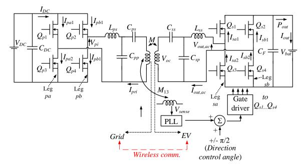
Fig. 2.14: A bidirectional DWPT system circuit diagram.
