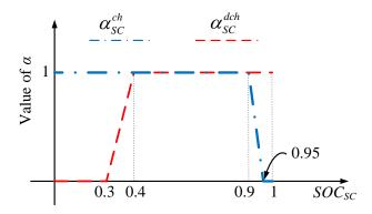
Fig. 5.22: SC current-derating factor vs. SOC.
