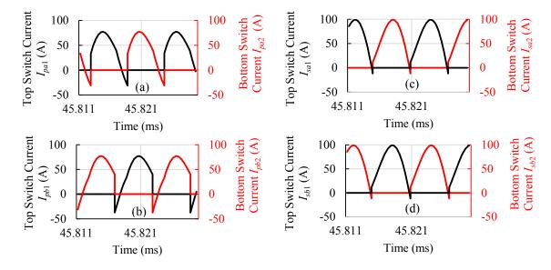
Fig. 4.25: Typical inverter switch currents for (a) leg pa and (b) leg pb, and rectifier switch currents for (c) leg sa and (b) leg sb while supplying the rated power of 25 kW to an EV.
