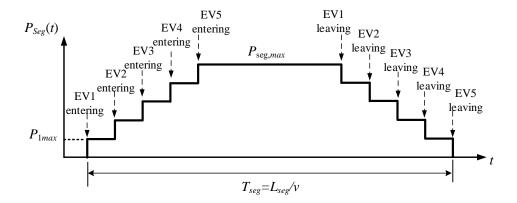
Fig. 2.7: The input power profile of one segment.
