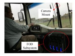
Fig. 3.25: (a) FOD system hardware (b) FOD system experimental setup mounted on the E-bus.
