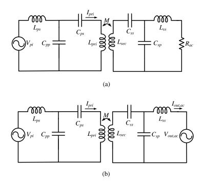
Fig. 2.10: Simplified equivalent WPT circuit with (a) resistive load model (b) battery load model.
