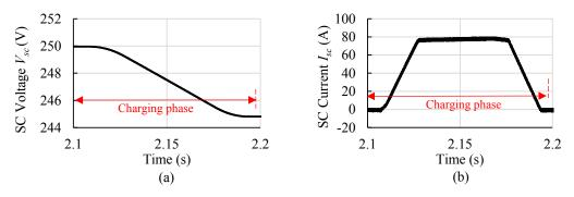
Fig. 4.36: (a) SC voltage  $V_{sc}$  and (b) SC current  $I_{sc}$  during the *charging phase* in G2V operation with bang-bang type control action of the *grid current controller*.
