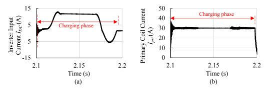
Fig. 4.37: (a) The grid current  $I_{DC}$  and (b) the primary coil current  $I_{pri}$  (RMS value) during the *charging phase* in G2V operation with bang-bang type control action of the *grid current controller*.
