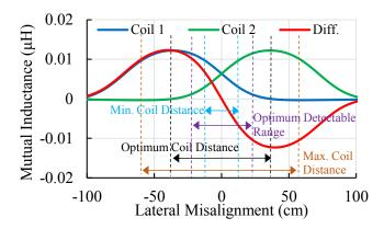
Fig. 3.12: Optimum operating zone location for a double-coil system.
