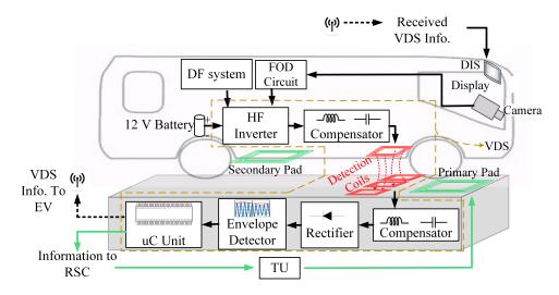
Fig. 3.1: Proposed DWPT system's operational block diagram with integrated DWPT-VDS.
