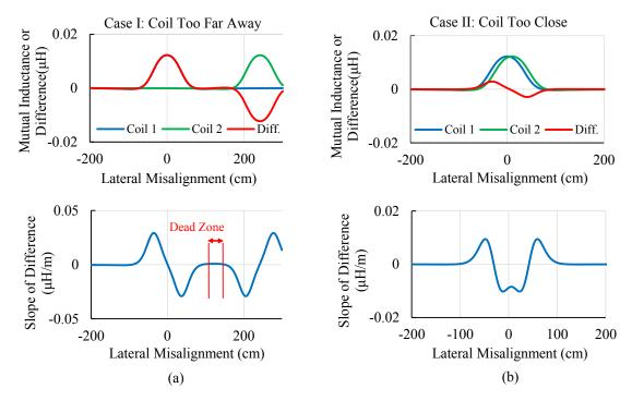
Fig. 3.10: The effect of distance between two coils of a double-coil design.
