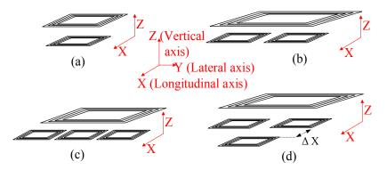
Fig. 3.6: (a) single-coil design (b) double-coil design (c) inline three-coil design and (d) triangular three-coil design.
