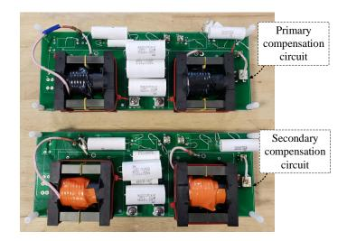
Fig. 4.58: Compensation circuits for the hardware prototype.
