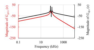
Fig. 4.9: Magnitude Bode plots of transconductances  $\frac{I_{pri}}{V_{pi}}$  and  $\frac{I_{Lps}}{V_{pi}}$ .
