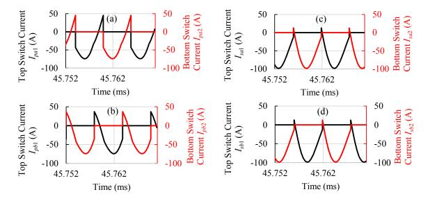
Fig. 4.27: Typical inverter switch currents for (a) leg pa and (b) leg pb, and rectifier switch currents for (c) leg sa and (b) leg sb while supplying the rated power of 25 kW to the grid.
