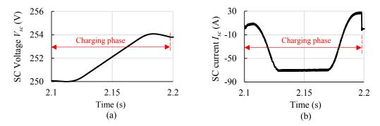
Fig. 4.40: (a) SC voltage  $V_{sc}$  and (b) SC current  $I_{sc}$  during the *charging phase* in V2G operation with FFFB type *grid current controller*.
