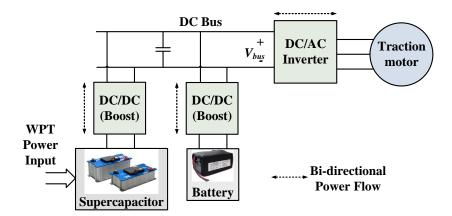
Fig. 5.8: Proposed HESS for DWPT-charged EV applications.
