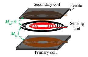
Fig. 4.55: The sensing coil structure configuration.
