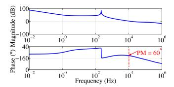
Fig. 5.19: Magnitude Bode plot of battery-converter compensated loop gain.
