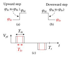
Fig. 4.14: (a) A step-up change in  $\phi_p$  (b) a step-down change in  $\phi_p$  (c) superimposed inverter outputs corresponding to two different conduction time periods resulted from the step change of (a) or (b).
