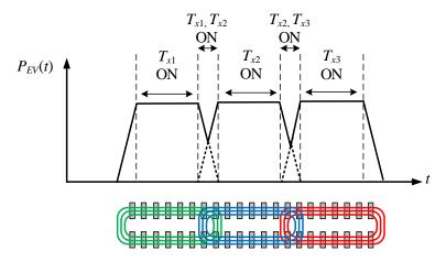
Fig. 2.4: Power transfer profiles from overlapped, sequentially-activated pads.
