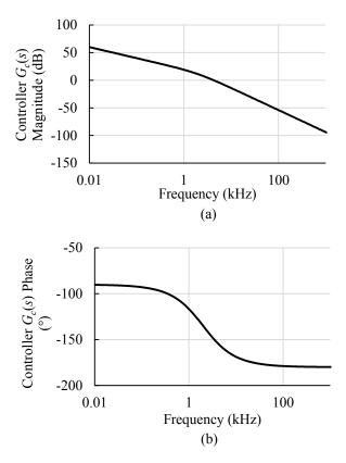
Fig. 4.17: Bode plots of the controller transfer function  $G_c(s)$ .
