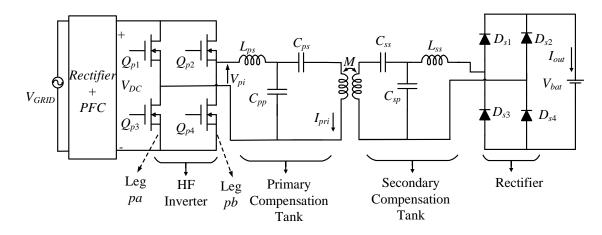
Fig. 2.8: A typical circuit for DWPT-charging of EVs.
