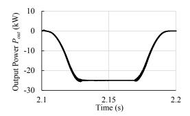
Fig. 4.39: The output power  $P_{out}$  profile during the charging phase in V2G operation with FFFB type grid current controller.
