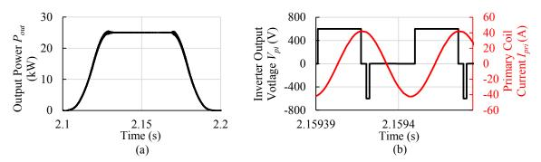
Fig. 4.34: (a) The output power  $P_{out}$  profile during the *charging phase* in G2V operation (b) the inverter output voltage  $V_{pi}$  and the primary coil current  $I_{pri}$  waveforms at one point during the *charging phase* with FFFB type control action of the *grid current controller*.
