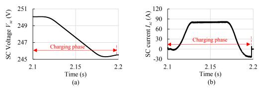
Fig. 4.35: (a) SC voltage  $V_{sc}$  and (b) SC current  $I_{sc}$  during the *charging phase* in G2V operation with FFFB type control action of the *grid current controller*.
