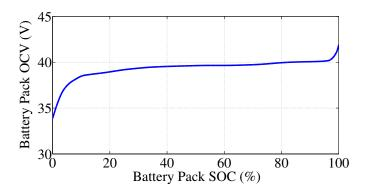
Fig. 5.4: Battery characteristic curve.
