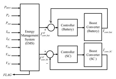
Fig. 5.21: EMS block diagram.
