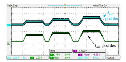
Fig. 4.70: Different G2V power profiles.
