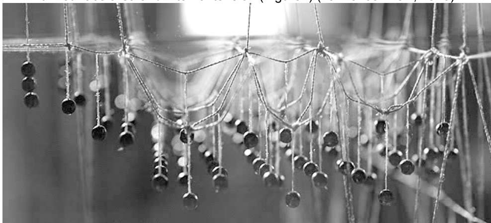
Figure 3 : Gaudí's experimental hanging model for finding the optimized form of structure in Sagra da familia Basilica (Burry, 1988)
