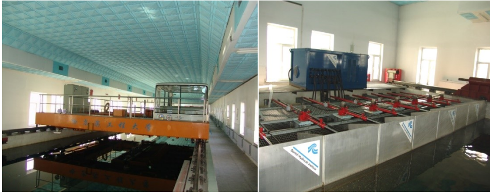
3 4 Fig.12. Wave tank, trailer, and wave maker at Harbin Engineering University.
