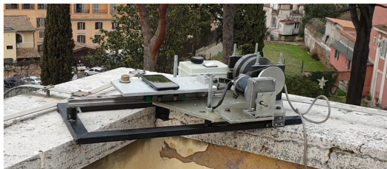
Figure 3. Vibrating table used to perform the tests.
