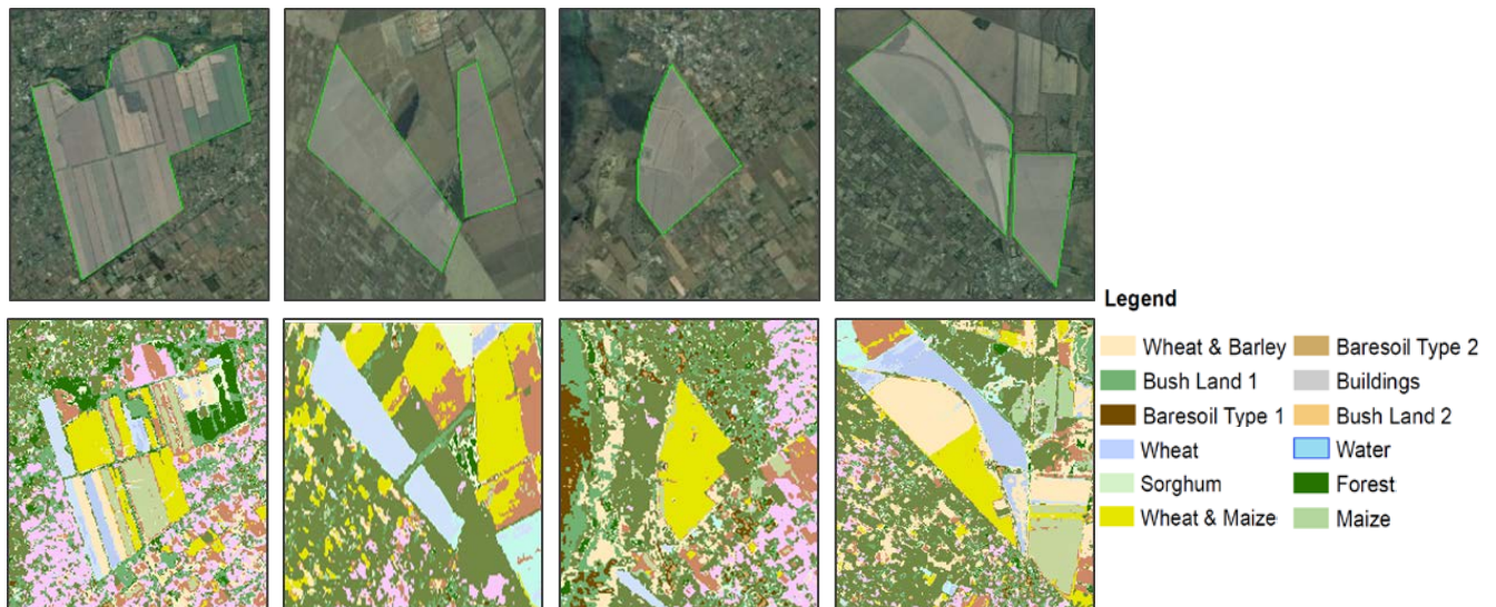
Figure 6. Crop boundaries representation: validation sites from Nakuru County (above); LULC maps of the same areas developed applying the here proposed methodology (below).
