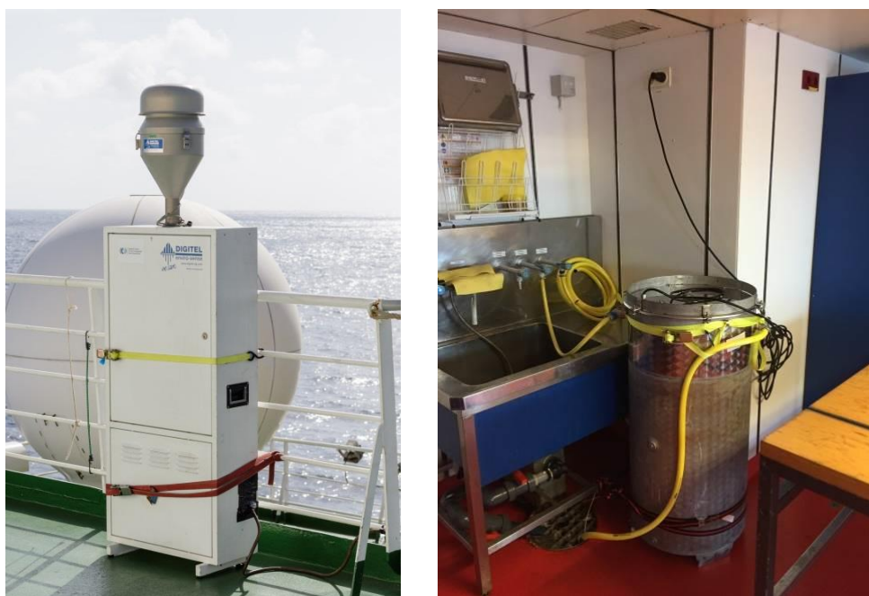
Figure 5.1.7.1 a) High-volume air sampler DH-77 at the 3 rd superstructure deck. b) 200L barrel for seawater sampling.
