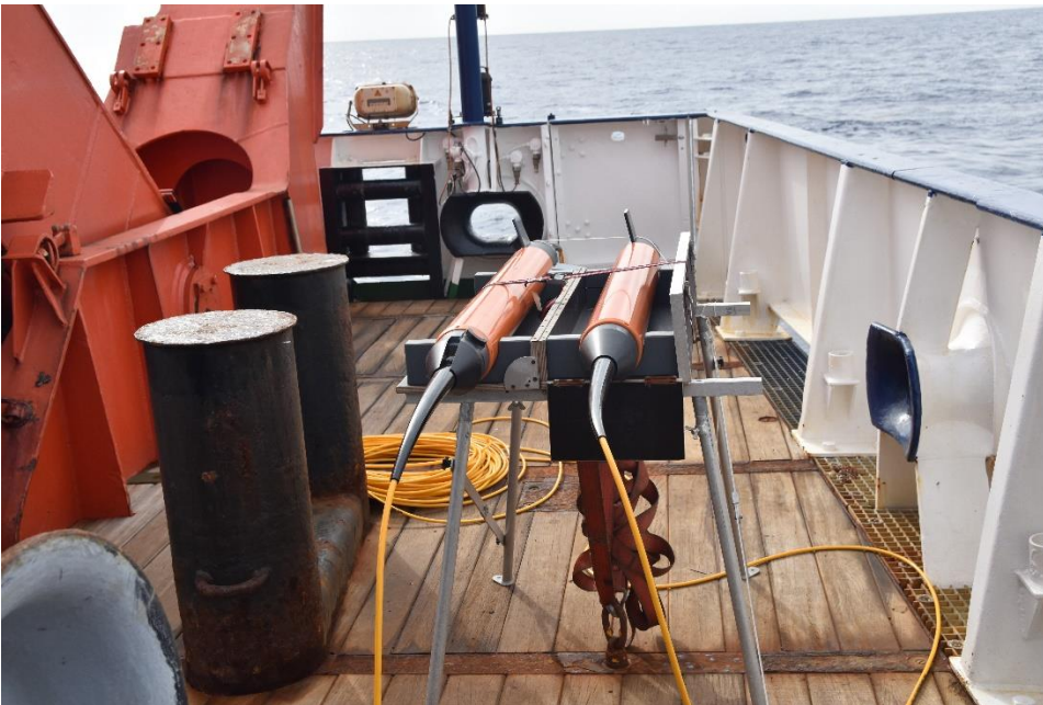
Fig. 12.2.4 Magnetic towfishes and connection cable ready for operation.
