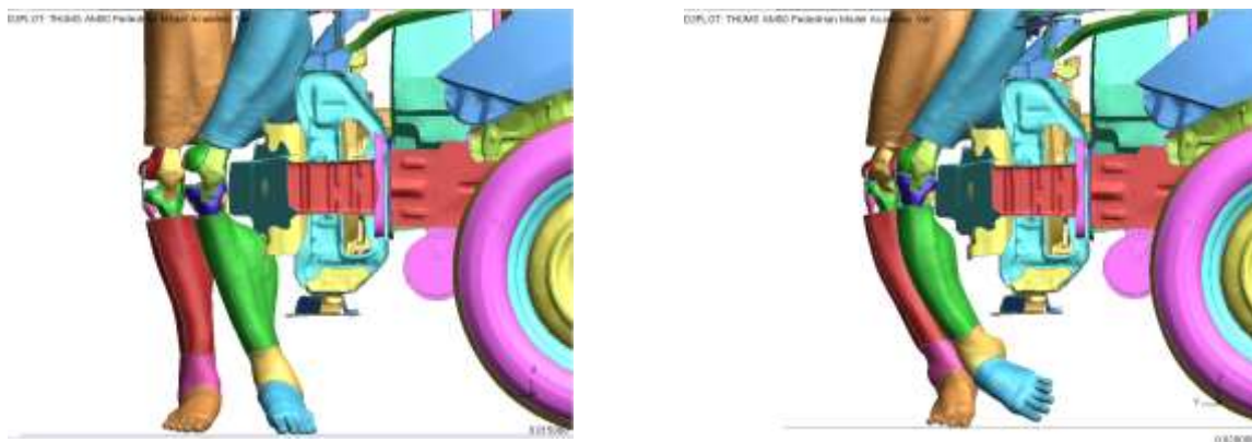
Fig.11: Femur separation from tibia and meniscus - original (Left) - after tendon material modifications (Right)
