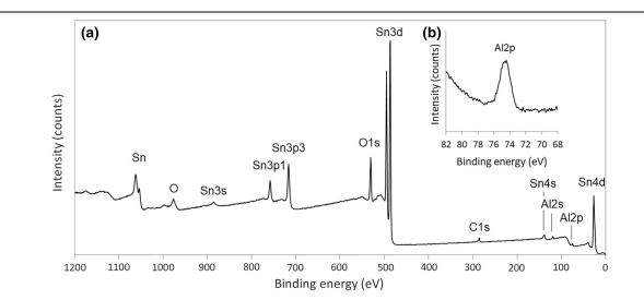
Fig. 13. XPS analysis showing the presence of AI on the surface of a thermally processed sample from batch 13: (a) survey scan and (b) high resolution scan of the Al2p peak.
