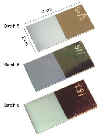
Fig. 3. Photograph showing the dimensions and appearance of selected ALD coated test coupons.
