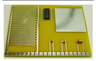
Fig. 14. Photograph showing the test board used to measure surface insulation resistance (SIR).
