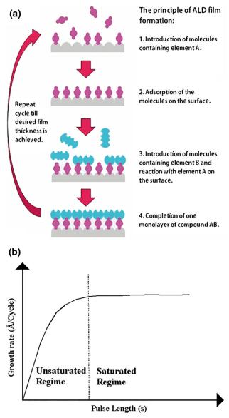
Fig. 2. ALD of a binary compound A-B using self-limiting surface chemistry: (a) reaction sequence with molecules containing elements A (e.g. Al) and B (e.g. O) and (b) saturation of growth rate with sufficient precursor pulse length. Figure courtesy of Picosun/Dr T. Suntola.
