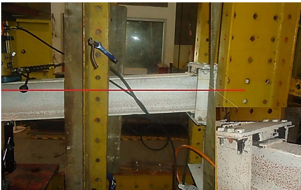
Figure 10. Damage state of the isolated connection
