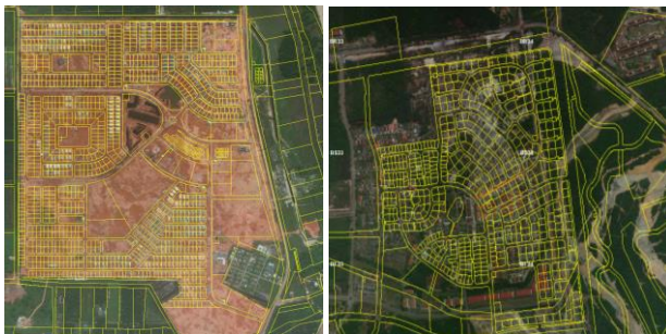
Figure 3: Example of correctly assigned (left) and slightly moved (right) land parcels based on satellite imagery validation
