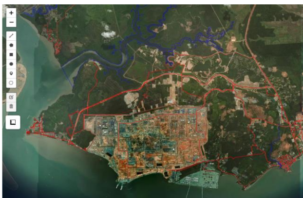
Figure 13: Multiple vector overlay (river and road) on top of online satellite imagery.
