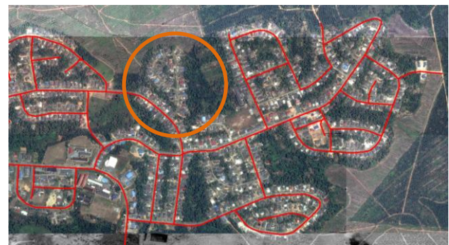
Figure 5: Example of correct road alignments from Open Street Map (OSM) but with missing data (orange circle)
