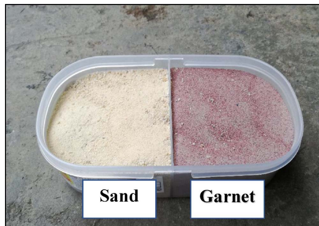
Fig. 1. Appearance of fine aggregates (sand and garnet) used in the concrete production.
