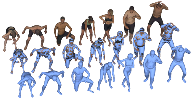
Fig. 1: Sample fitting results of BODYFITR on challenging poses of 3DBodyTex [1] with scan (back), fitted model (front) and overlay (middle).
