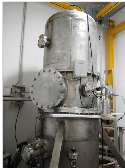
Figure 1: the Chambre structure: a 7-stage Andersen impactor for bioaerosol collection is visible on the right side
