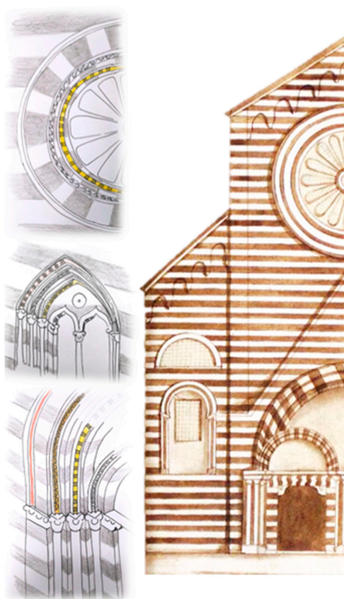
Figure 8. Inferred appearance of the façade, according to the data that emerged in the present study. On the left side, reconstructions of the decorative reliefs of a rose window, double arched windows and a splayed portal, and their colours. The possible positioning of the analysed fragments on the façade, along with its chromatic scheme, based on the paint relics is rendered with three virtual models. On the right hand side, for comparison, a reproduction of the drawing of the façade from the manuscript Epitaphia, sepulcra et inscriptiones cum stemmatibus marmorea et lapidea existentia in ecclesiis genuensibus , by Domenico Piaggio, folio 12, courtesy of the Berio Library, Genoa.
