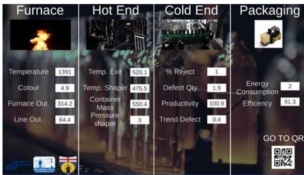
Figure 3: Mobile application displaying main plant indicators
