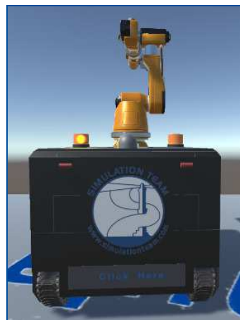
Figure 4 – UGV with arm to perform task in Industrial Plant under development by Simulation Team
