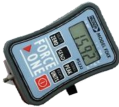
Figure 4. The Pressure Gauge used for this study, a Wagner Instruments FDIX Force One pressure algometer (Wagner Instruments, Greenwich, CT)
