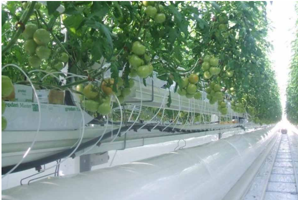
Figure 7 Weighing gutter for automated monitoring of crop evapotranspiration and irrigation control in tomato substrate culture. The suspended trough with some tomato plants is connected to a load cell: the difference in weight between two consecutive irrigations represents the crop evapotranspiration in this interval. Photo: A. De Koning, Hortimax, Pijnacker, NL.
