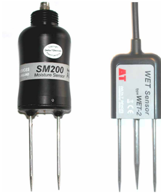
Figure 8 Two examples of dielectric sensors for measuring substrate water content: SM 200™ (left) and WET™ (right), both commercialized by Delta-T device Ltd (UK). The latter sensor also measures substrate salinity (bulk EC) and temperature.
