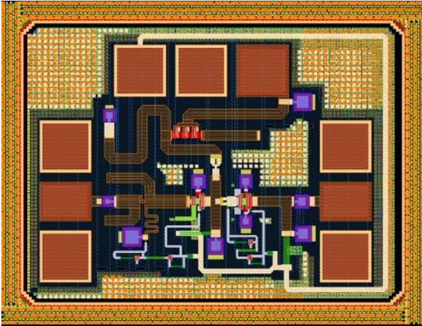
Fig. C.9. Momentum mask (left) and fabricated chip (right) of the LNA design using a HBT-RF switch (Chapter 6).
