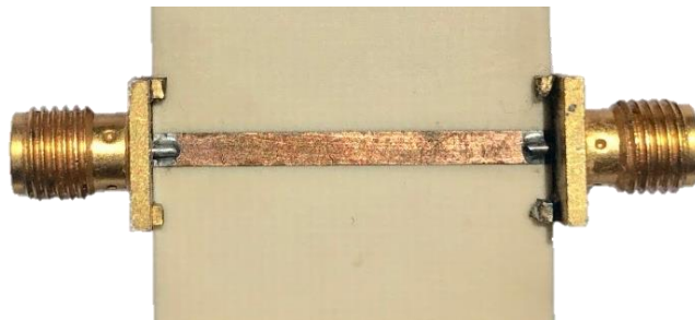
Fig. 4.15. Coaxial connectors and the fabricated microstrip line.
