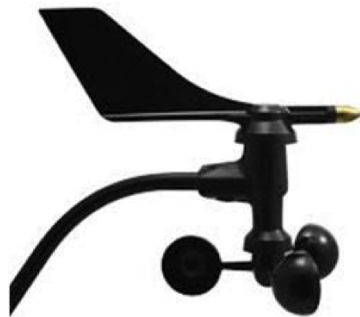
Figure 5.37. Davis Cup anemometer.
