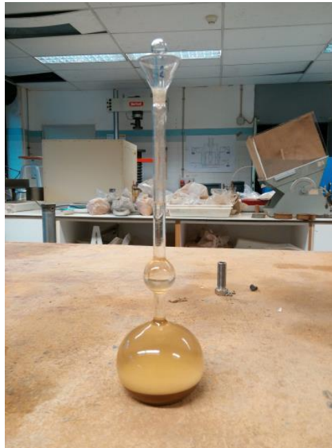
Figure 5.8. Pycnometer used to determine specific gravity.
