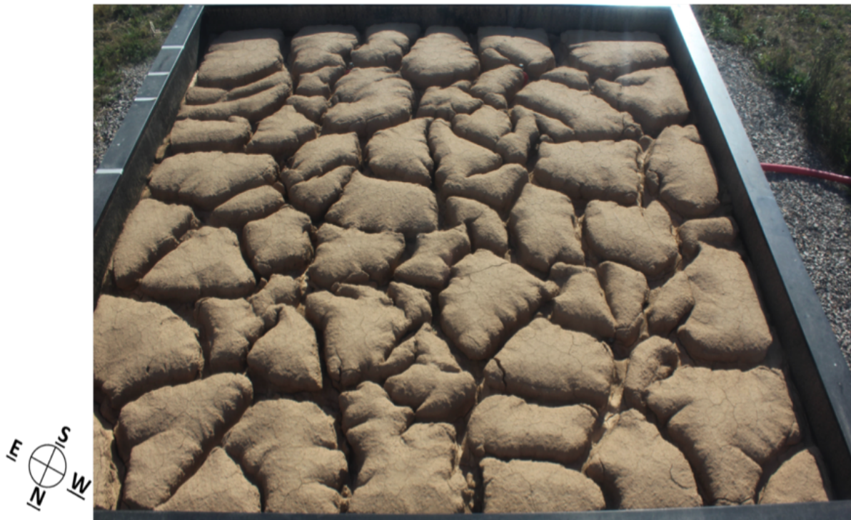
Figure 5.84. Specimen surface at the conclusion of the one-year test on 17-Jan-2016.
