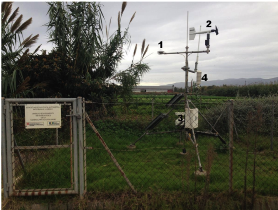
Figure 5.27. Viladecans automatic weather station. 1) pyranometer; 2) anemometer and vane ; 3) pluviometer; 4) capacitive hygrometer and thermistor.
