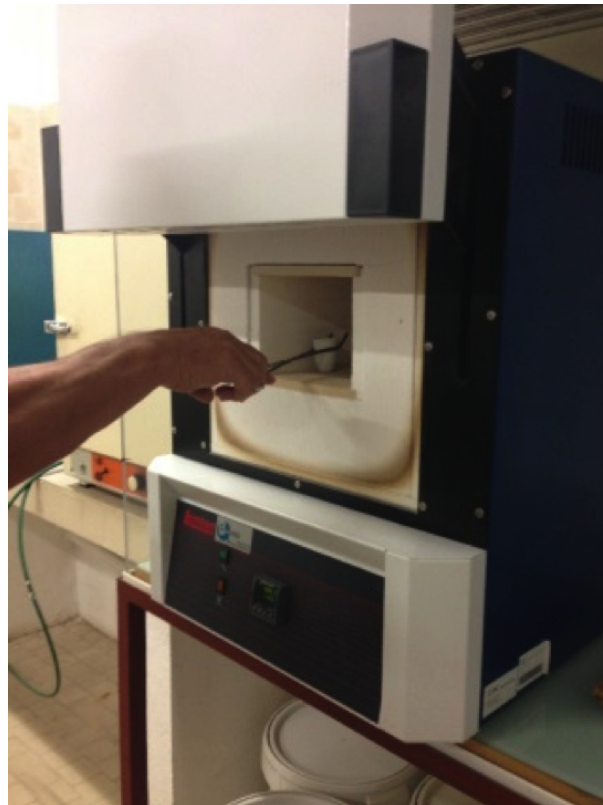
Figure 5.14. Organic matter determination in a muffle furnace.
