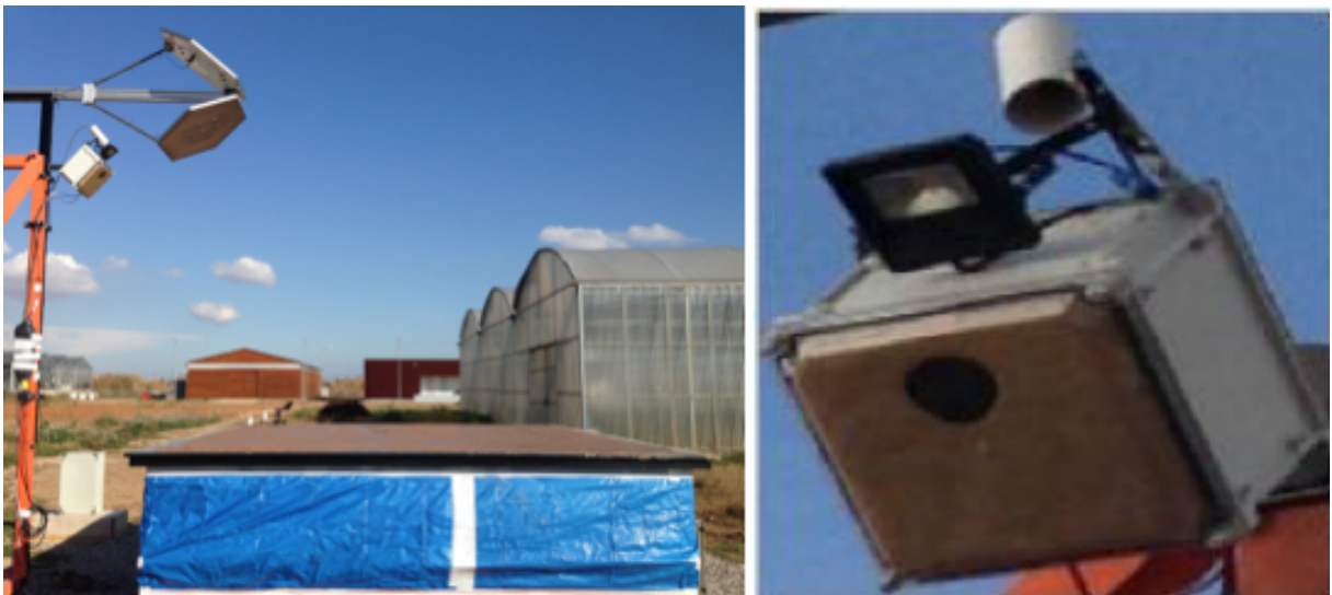
Figure 5.39. Surface image capture equipment adapted for the field test.
