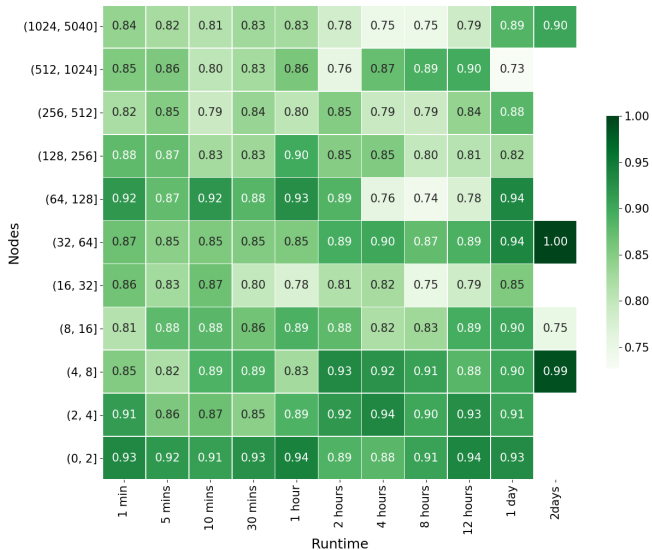
Figure 5: Heatmap showing the ratio between run time of static backfill and SD-Policy MAXSD 10 using workload 4, for different job categories.
