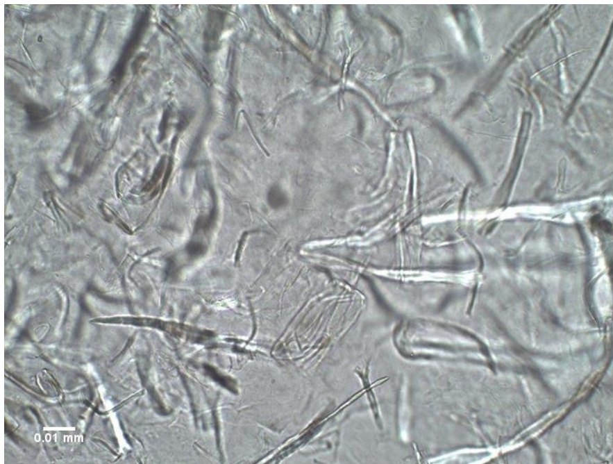
Figure 10. Picture of 1wt% hydrogel displaying CNFs appearance at 15,625 magnifications.
