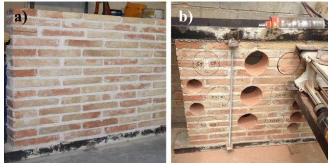
Fig. 1. a) Masonry wall built in the laboratory for the campaign “MA”, and b) core drilling of 150 mm and 90 mm cylindrical samples.
