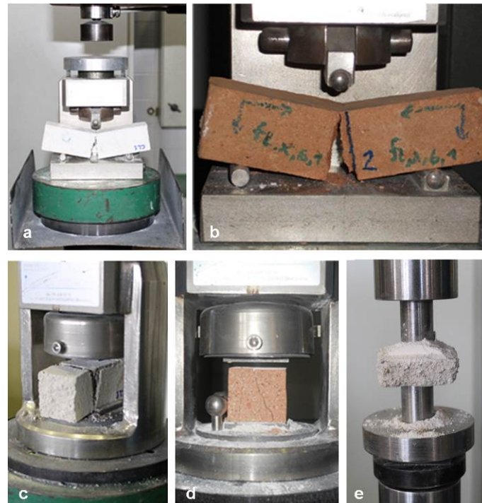
117 Figure 1 – Flexure and compression testing of prismatic samples of mortar (a,c) and brick (b,d). Double 118 punch testing of mortar joints (e).
