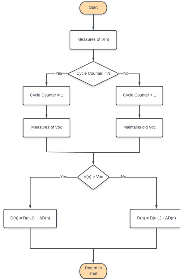
Figure 5.7: Flowchart: Open-Circuit voltage algorithm
