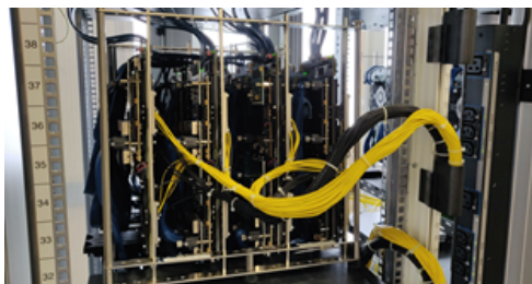
(a) Cluster of 4 motherboards representing an HN node placed on a rack
