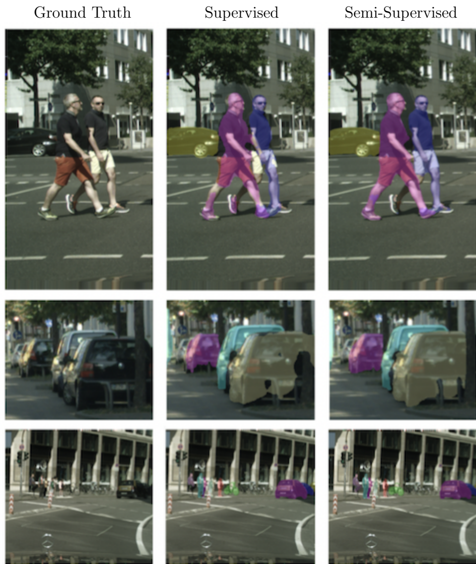
Figure 5.5: Some examples of the results obtained on the Cityscapes Dataset. Left: Ground Truth, Center: Supervised Network on 10% of the data. Right: Predictions with our semi-supervised method.
