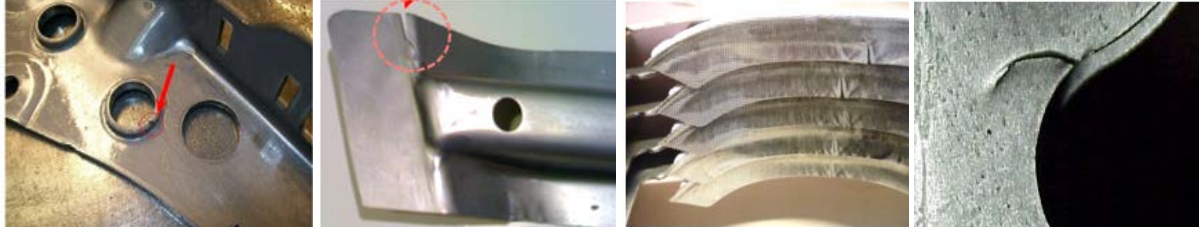
Figure 1. Examples of edge cracking in cold formed components
