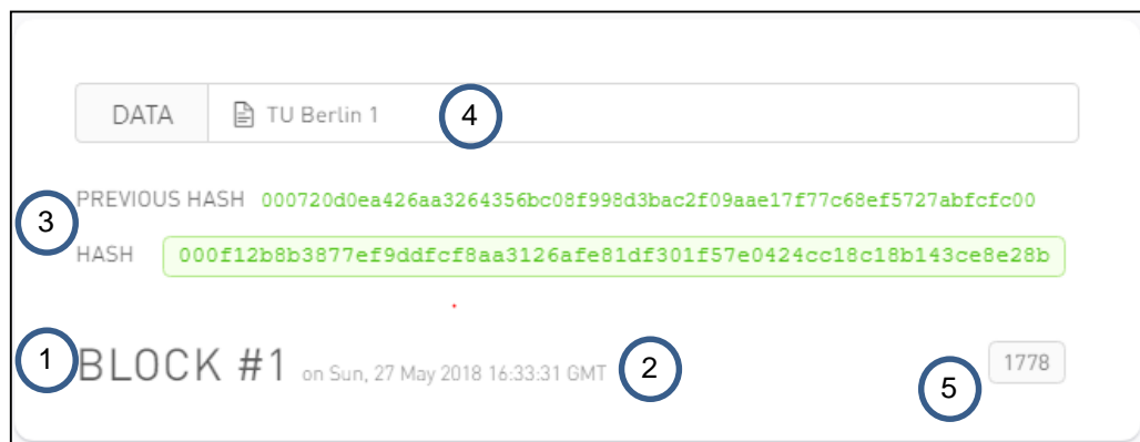
Figure 3: Block example: (1) Index, (2) Timestamp, (3) Previous and Current Hash, (4) Data input, (5) Nonce.
