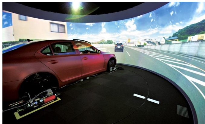
Figure 19: Lexus VR driving simulator. Source: Lexus. Retrieved from Hypergrid Business. (29, October 2015). 75% of top brands have VR projects
