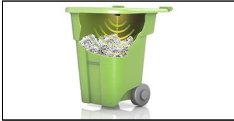
Figure 30 Sensor in a garbage container 41
