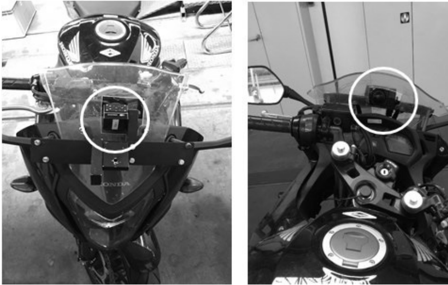
Figure 22: Front camera fixing
