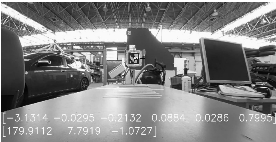
Figure 34: Detected marker with coordinates
