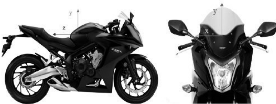
Figure 9: Coordinate system in the motorbike
