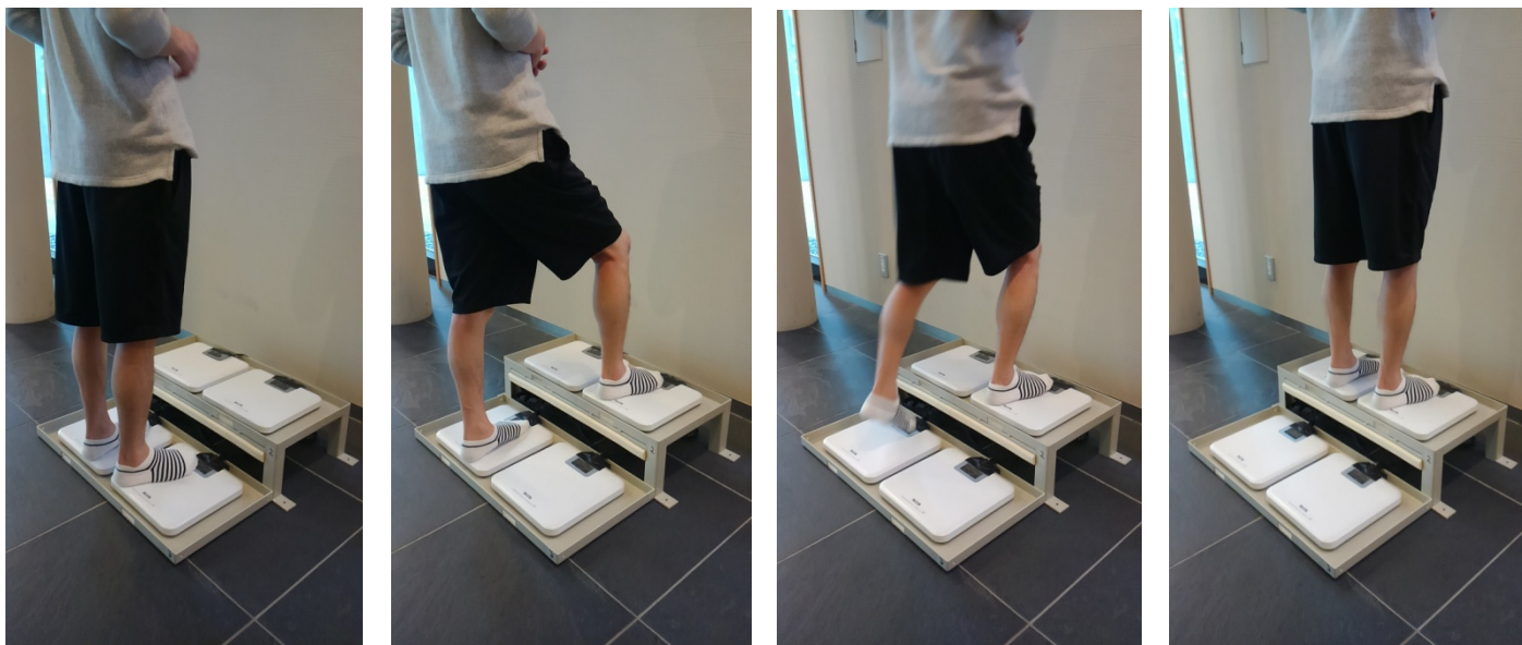
FIGURE 1. Step ascent motion measurement on a step ascent platform.
