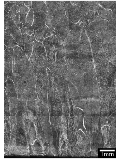
Fig. 12. As-cast \gamma grain structure in the sample with 0.015 wt% P obtained from the permanent mold casting experiment. The top and the bottom of the micrograph correspond to the center of the ingot and the sidewall surface, respectively.
