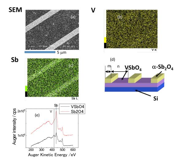
Figure 1 SEM, EDX images and spot auger spectraof the-  $\alpha$ -Sb<sub>2</sub>O<sub>4</sub>/VSbO<sub>4</sub> thin film L100S400. (a) Secondary electron image, and (b) V K $\alpha$ , and (c) Sb L $\alpha$  fluorescence images. (d) Schematic of the sample structure.(e) spot Auger spectra of VSbO<sub>4</sub>(black solid line) region and  $\alpha$ -Sb<sub>2</sub>O<sub>4</sub> region(red dotted line).
