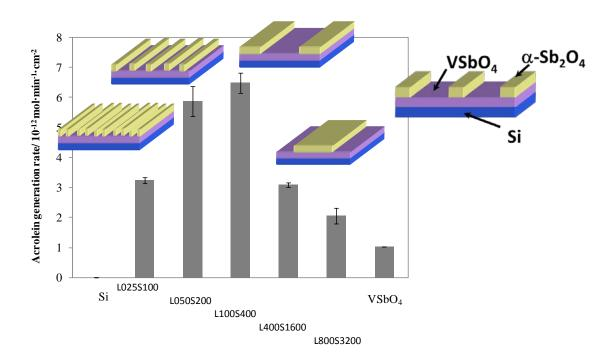
Figure 2 Generation rates of acrolein from propene oxidation (523 K, 0.2 Pa propene, 0.2 Pa  $O_2$ , 0.6 Pa Ar) on precisely designed  $\alpha$ -Sb<sub>2</sub>O<sub>4</sub>/VSbO<sub>4</sub>/Si catalysts with different ribbon separation values but the same ratio of ribbon separation to width of 4:1 (L025S100, L050S200, L100S400, L400S1600, and L800S3200). The generation rates of VSbO<sub>4</sub>/Si, and a Si substrate were give for reference.
