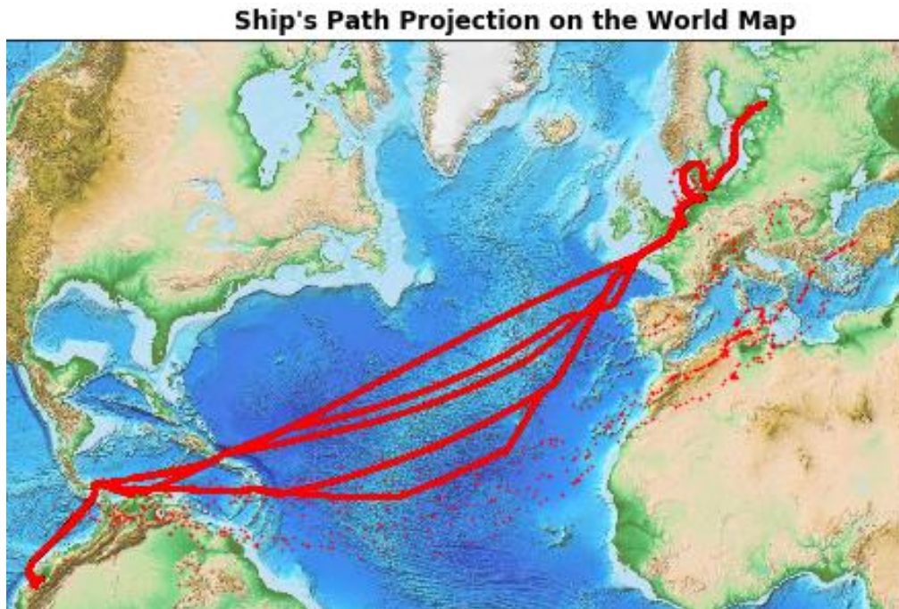
Figure 3.15 The latitude and longitude coordinates as acquired from the GPS on-board the ship. Raw-data map projection.
