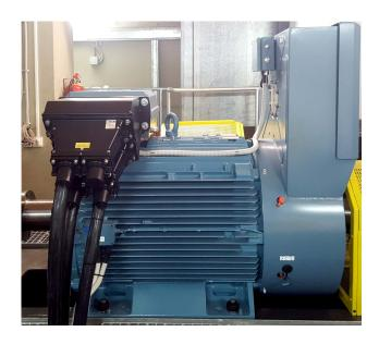
Figure 2.6: ABB Electric Brake 315 kW.
