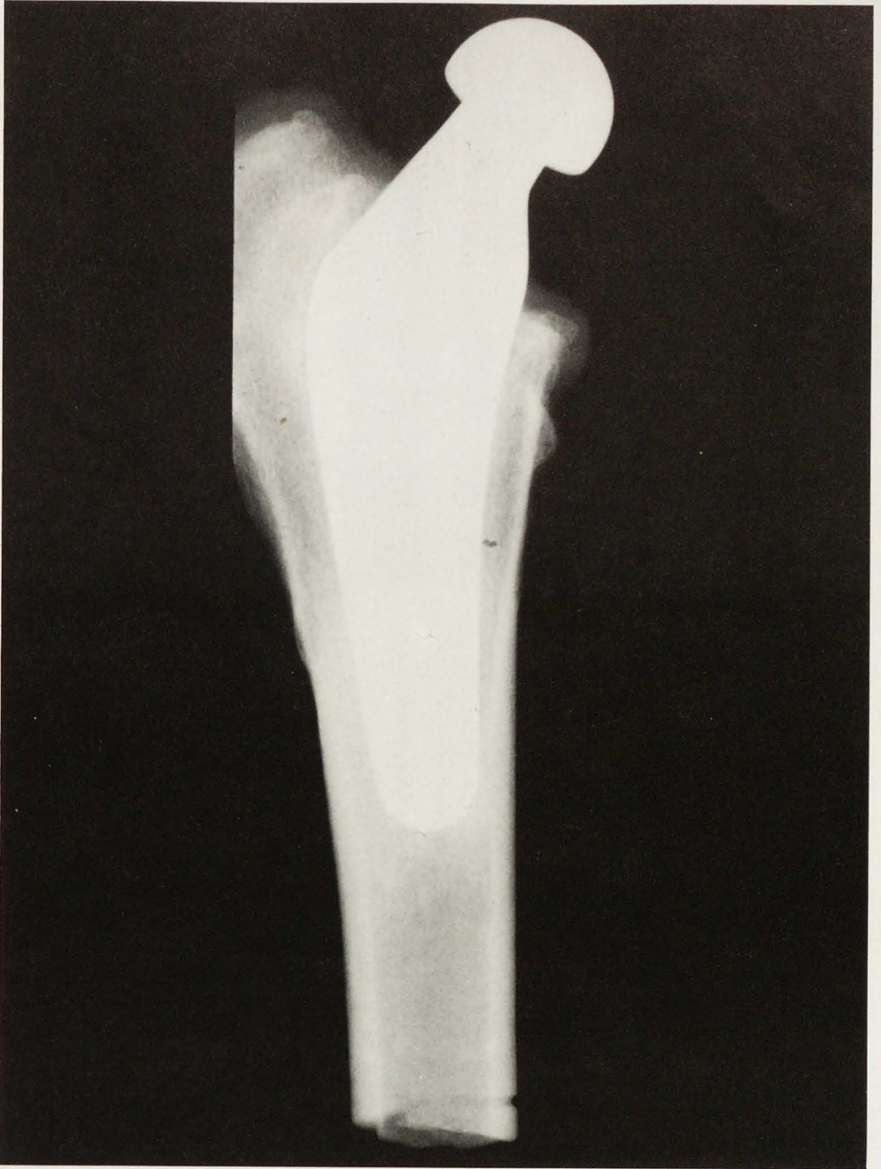
Fig. 52 Bone densification around hydroxyl-apatite coated implants is especially evident in proximal and distal stem area at one year follow-up. Moderate loss of cortical wall thickness in proximal femur (AP explant radiograph).
