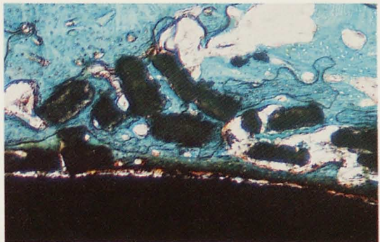
Fig. 90 Severe fragmentation of infected hydroxyl-apatite coating at interface of coated femoral stem (Masson-trichrome, six months, x200).
