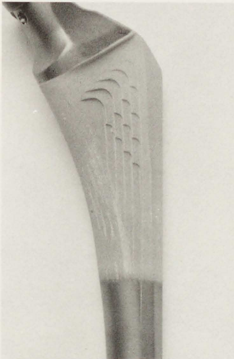
Fig. 13 Retrieved femoral stem after cadaver implantation.
