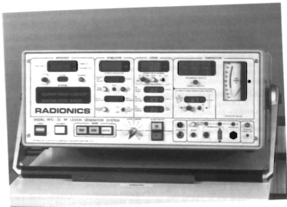
Figure 1. Radiofrequency lesion generator Radionics 3C with following functions: impedance monitor, stimulator, lesion parameters and temperature monitor.
