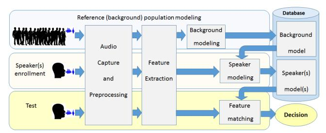
Figure 10: Schematics of a speaker recognition system.
