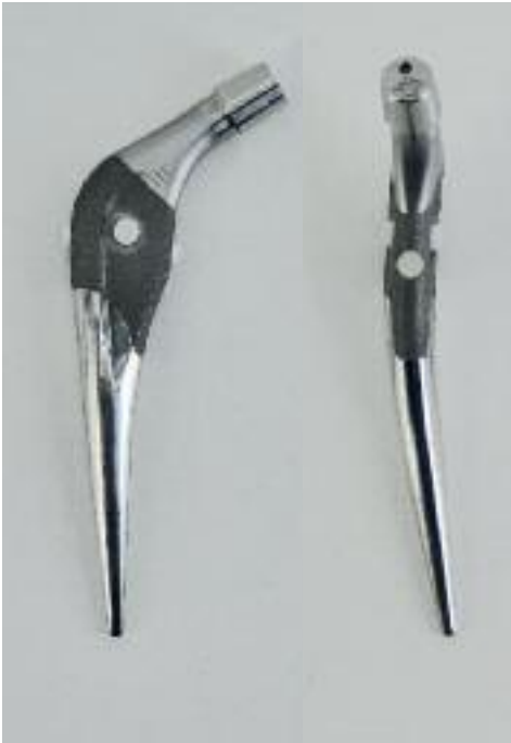
Fig. 2 AP and Lat view of the collarless anatomically shaped SHP stem with PMMA cement spacers (distal spacer not shown). Proximally a rigid part with rough surface finish ( R_a=3.8 \mu\text{m} ), distally a flexible taper with polished surface ( R_a0.05 \mu\text{m} ). Reinforcement profile at the lateral side of the stem to resist bending forces and to reduce subsidence risk.
