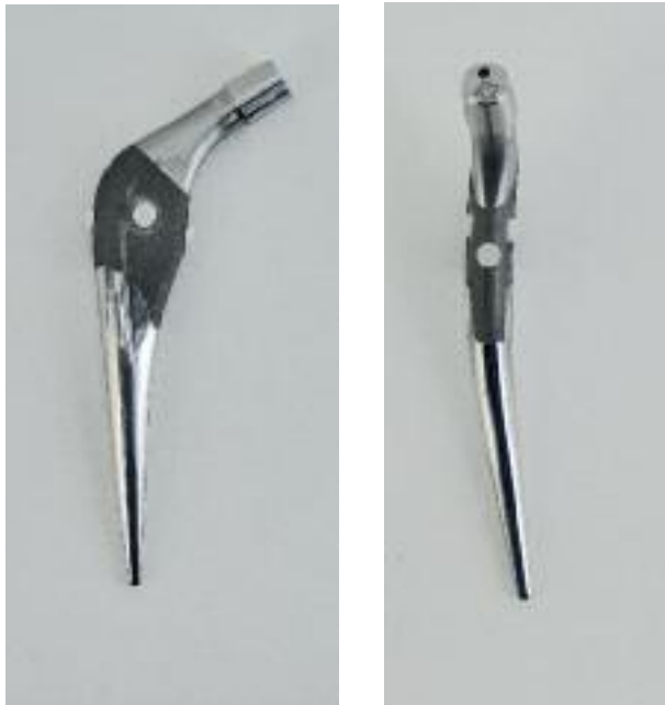
Fig. 1a AP and Lat view of the collarless anatomically shaped SHP ® stem with PMMA cement spacers (distal spacer not shown) to guarantee a minimal cement thickness of 2 mm. Proximally it shows a rigid part with rough surface finish ( R_a=3.8 \mu\text{m} ), distally it has a flexible taper with polished surface ( R_a<0.05 \mu\text{m} ) to prevent abrasive wear in case of debonding
