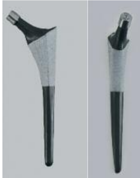
Fig. 2 Illustrations of the Symax™ stem in AP (left) and lateral (right) view, showing a straight stem with the neck in an anteverted position. It features a proximal plasma-sprayed CP Titanium layer, with a biomimetic electrochemically deposited BONIT®-HA coating of very high porosity of 60%, and only 10-20 µm thick. Distally the stem is treated with the Dotize® surface process, which reduces distal bone apposition and osseointegration.
