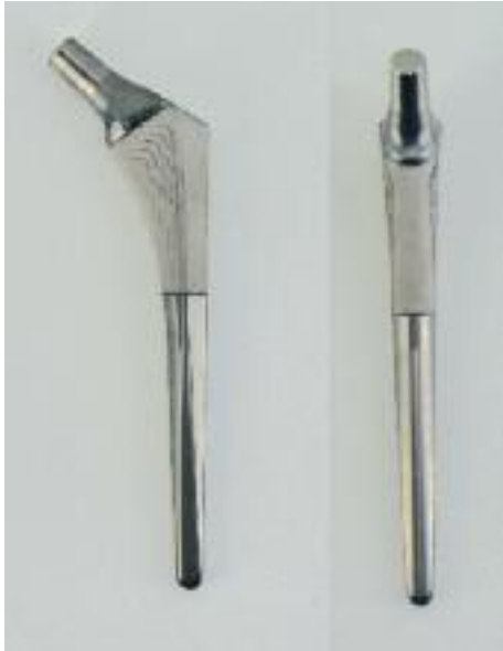
Fig. 1 The HA Omnifit® hip stem, geometrically a straight double wedge design, is made of Ti-alloy, has a macro-textured surface of which the proximal 40 % is plasma sprayed HA-coated, and has a distal matte finish, all aimed at proximal fixation. The HA-coating is highly crystalline (65%) explaining slow resorbability.
