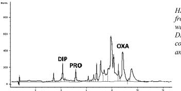
HPLC chromatogram from analysis of a surface water sample spiked with DIP, OXA and PRO at a concentration of 10, 20 and 10 µg/L, respectively.
